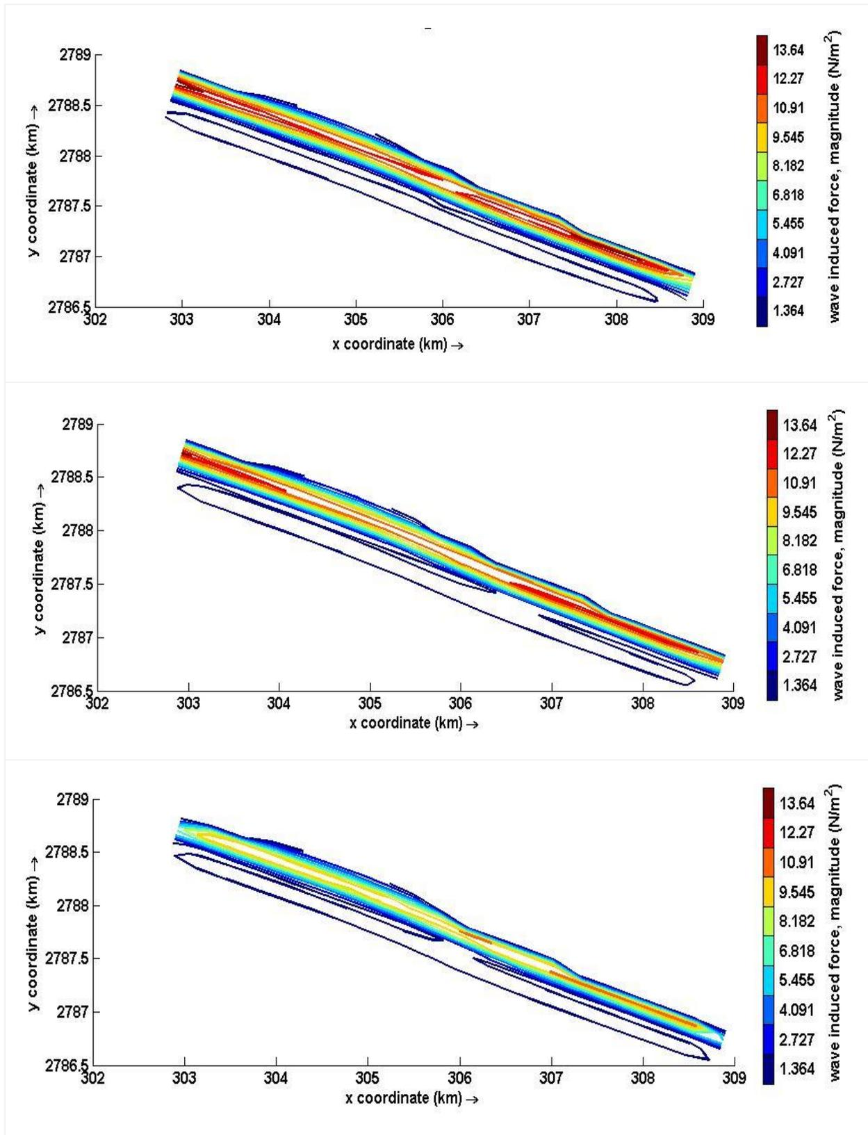
Fig. 7: Change in wave force in computational domain
