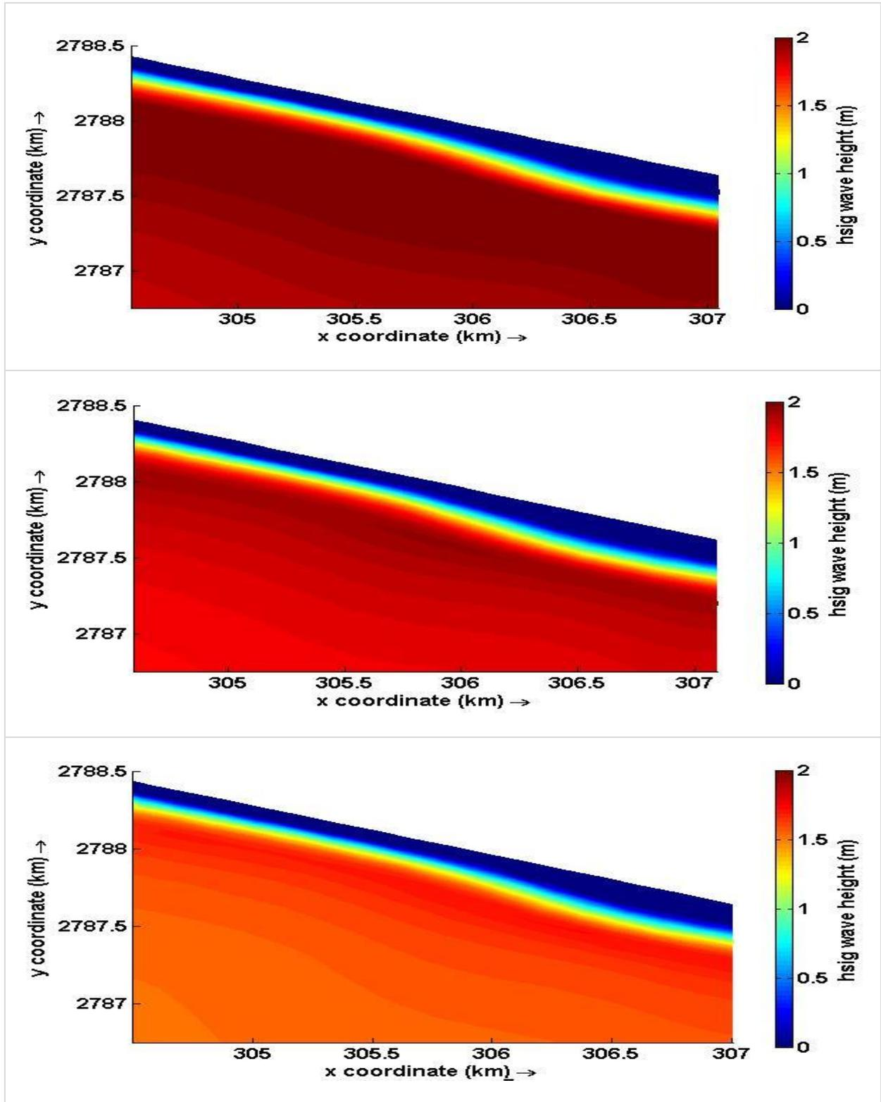
Fig. 6: Change in wave height in computational domain
