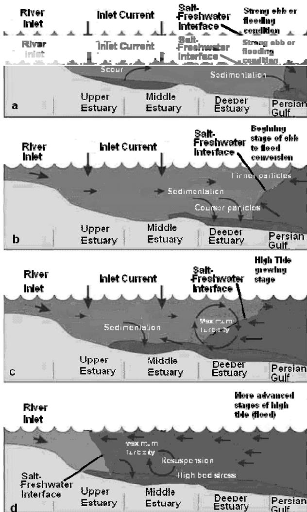
Fig 2. Schematic diagram of the tidal dynamics at the vicinity of Bahmansheer Estuary for four different stages; a-Strong ebb or flooding, b-Stage of ebb to Flood conversion, c-High tide growing stage (flood), d-Mature stage of flood (high tide)
