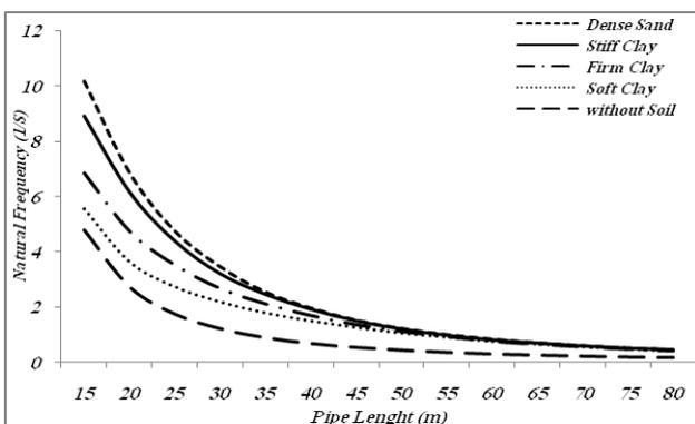
Fig. 10: Effect of seabed soil on the natural frequency in pinned-pinned boundary condition
