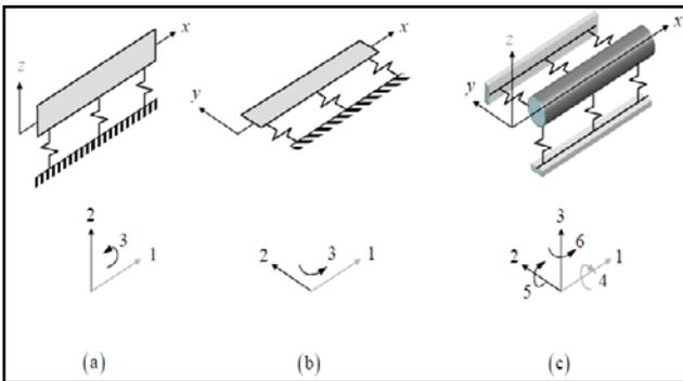
Fig. 3: Degrees of freedom of beam element in vertical plane (a), lateral plane (b) and in ABAQUS (c)
