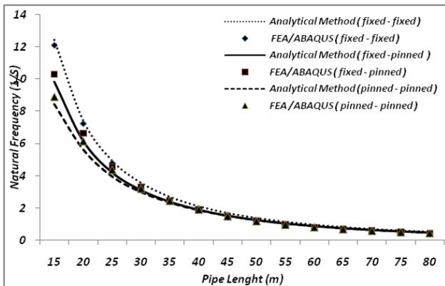
Fig. 16: Effect of dense clay on the natural frequency of pipelines
