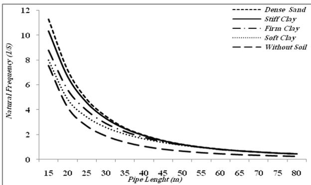
Fig. 9: Effect of seabed soil on the natural frequency in fixed-pinned boundary condition
