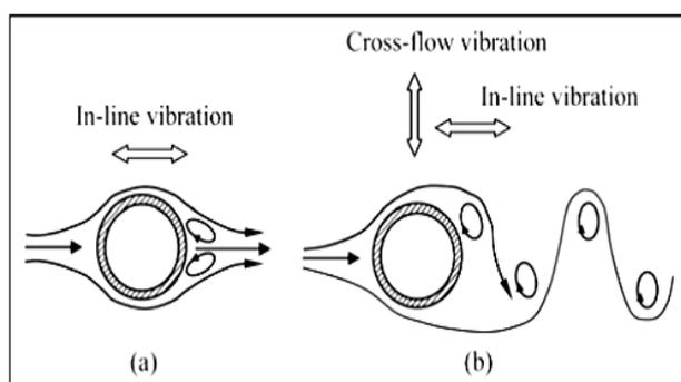
Fig. 2: Vortices and vibrations of free span section: (a) symmetrical vortices and in-line vibration; (b) asymmetrical vortices and in-line and cross-flow vibrations (Zhi-Gang Xiao et al., 2010)
