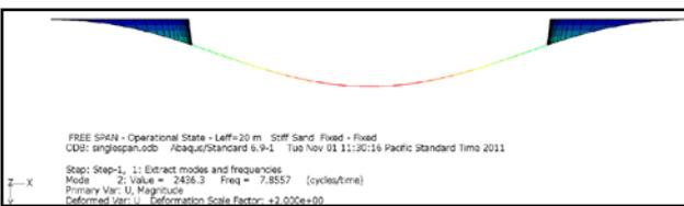
Fig. 11: The results of analysis in the ABAQUS software in fixed / fixed boundary conditions for the pipeline with length 20 m lay on seabed with the dense sand formation
