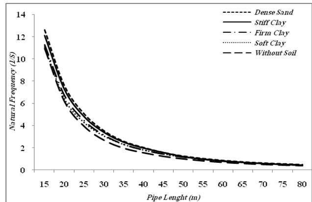
Fig. 8: Effect of seabed soil on the natural frequency in fixed-fixed boundary condition
