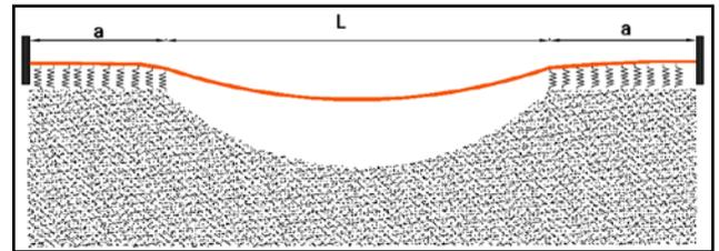
Fig. 4: A schematic representation of the free spanning of the pipeline on the seabed
