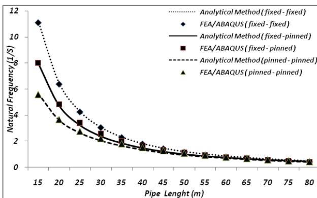
Fig. 18: Effect of soft clay on the natural frequency of pipelines
