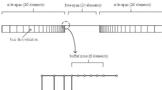
Fig. 7: Schematized illustration of mesh in the ABAQUS model for the single-span pipeline.
