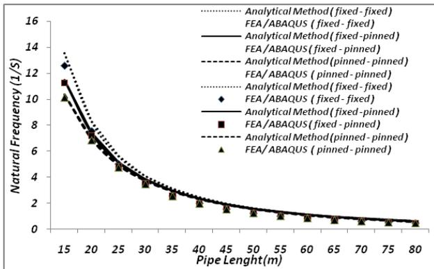
Fig. 15: Effect of dense sand on the natural frequency of pipelines
