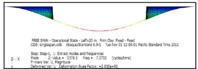
Fig. 13: The results of analysis in the ABAQUS software in fixed / fixed boundary conditions for the pipeline with length 20 m lay on seabed with the firm clay formation
