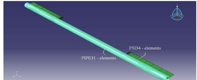
Fig. 5b: Elements in the ABAQUS Model
