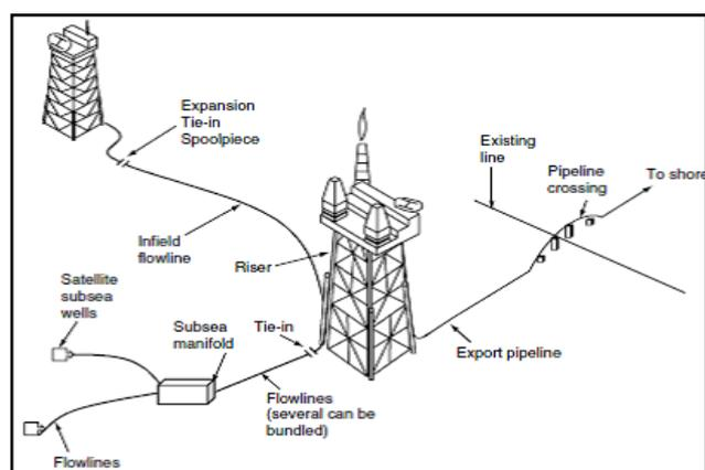
Fig. 1: Use of flow lines offshore pipeline (from Bai 2001)
