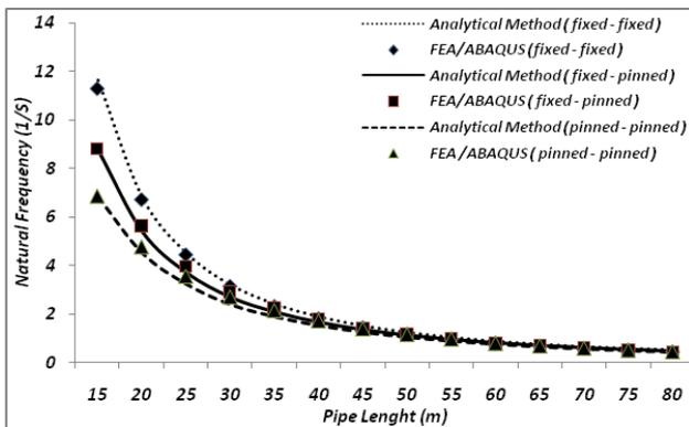
Fig. 17: Effect of firm clay on the natural frequency of pipelines
