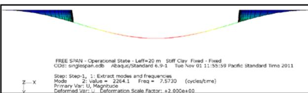
Fig. 12: The results of analysis in the ABAQUS software in fixed / fixed boundary conditions for the pipeline with length 20 m lay on seabed with the dense clay formation
