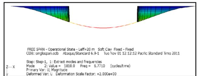
Fig. 14: The results of analysis in the ABAQUS software in fixed / fixed boundary conditions for the pipeline with length 20 m lay on seabed with the soft clay formation
