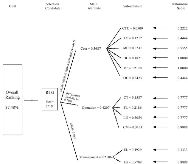
Fig. 5: The AHP value tree for RTG
