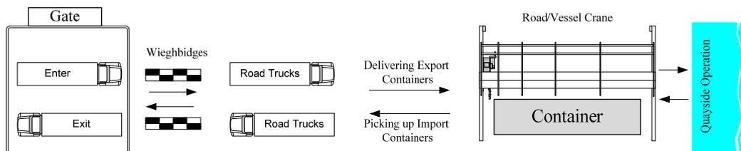
Fig. 2: Process of loading/discharging operation in a typical marine container terminal
