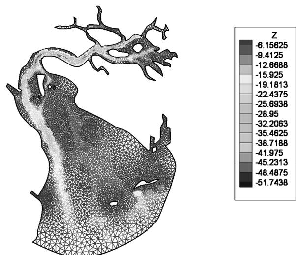
Fig 5. Unstructured triangular mesh including bed elevation data
