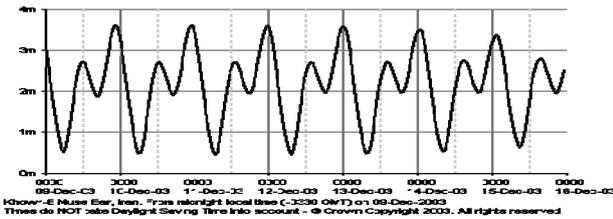
Fig 6. Water surface fluctuations imposed at far field boundaries of computational domain (predicted by the harmonic analyses data which is calibrated by Easy Tide Prediction)
