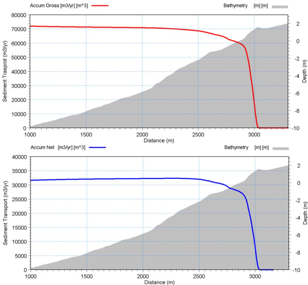
Fig 7: a: Cumulative sediment transport potential and cross section of bathymetry
