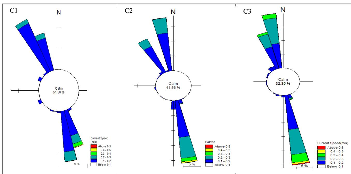
Fig 5: Current rose plot of data at 8m depth - C1: in front of Bonji port (north of the project site) – C2: in front of the project site – C3: in Kuhmobarak area (south of the project site)
