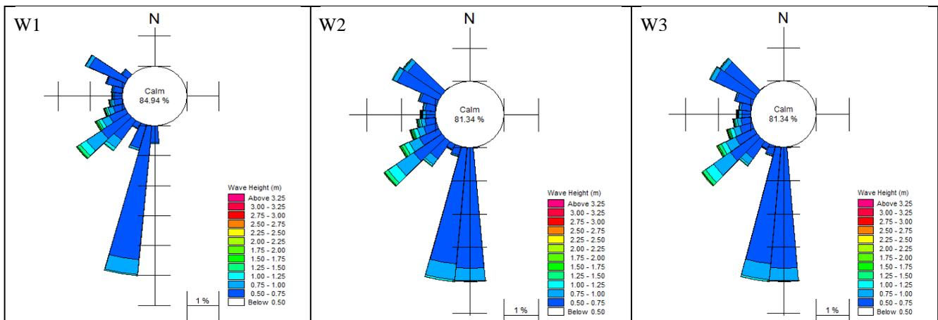
Fig 4: Waverose plot of data at 15m depth - W1: in front of Bonji port (north of the project site) - W2: in front of the project site - W3: in front of Kuhmobarak port (south of the project site)
