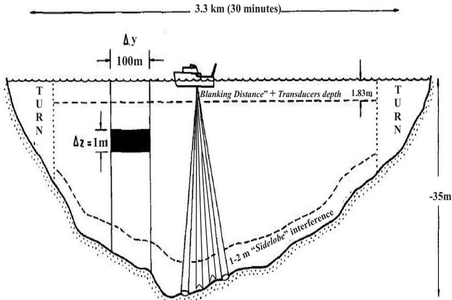
Fig. 2: Schematic of strategy for MV-ADCP measurements in which the boat repeatedly traversed the channel. There are no data available during turns at the end of each run and in near-surface and near-bottom sections of the profile.
