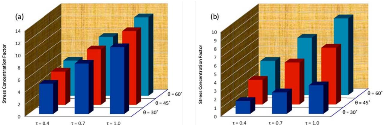
Fig. 4: Effect of the  $\tau$  on the SCF values at the saddle position under the 1st OPB loading condition ( $\beta = 0.6, \gamma = 12$ ): (a) Central brace, (b) Outer brace
