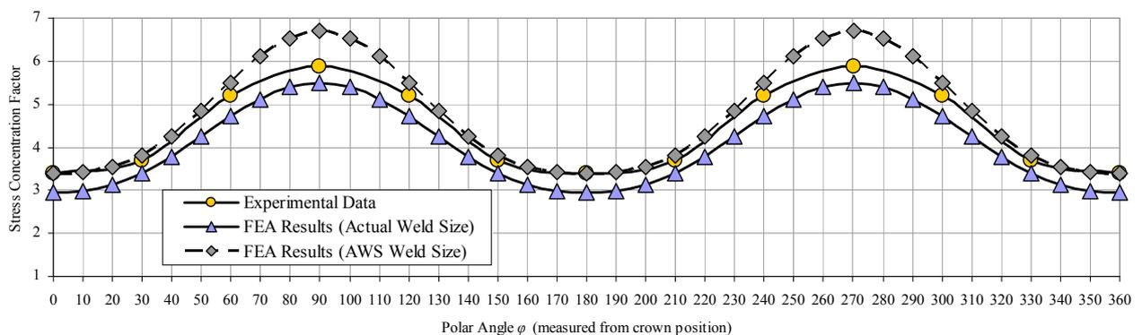
Fig. 3: Distribution of chord-side SCFs along the central brace/chord intersection of an unstiffened gap KT-joint: Comparing the results of experimental modeling and FE analysis
