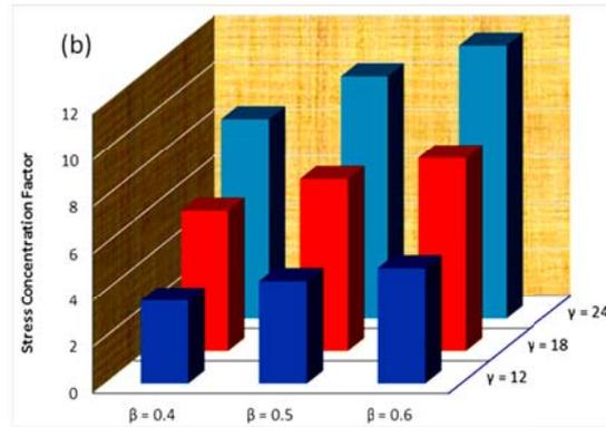
Fig. 5: Effect of the  $\beta$  on the SCF values at the saddle position under the 1st OPB loading condition ( $\tau = 0.7$ ,  $\theta = 45^\circ$ ): (a) Central brace, (b) Outer brace
