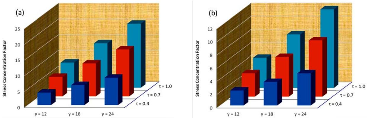
Fig. 6: Effect of the  $\gamma$  on the SCF values at the saddle position under the 1st OPB loading condition ( $\beta = 0.4$ ,  $\theta = 45^\circ$ ): (a) Central brace, (b) Outer brace
