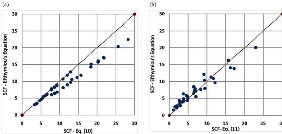
Fig. 8: Comparison of SCFs obtained from equations proposed by Efthymiou (1988) and present research – 1<sup>st</sup> OPB load case (Fig. 1d): (a) central brace chord-side SCFs; (b) outer brace chord-side SCFs
