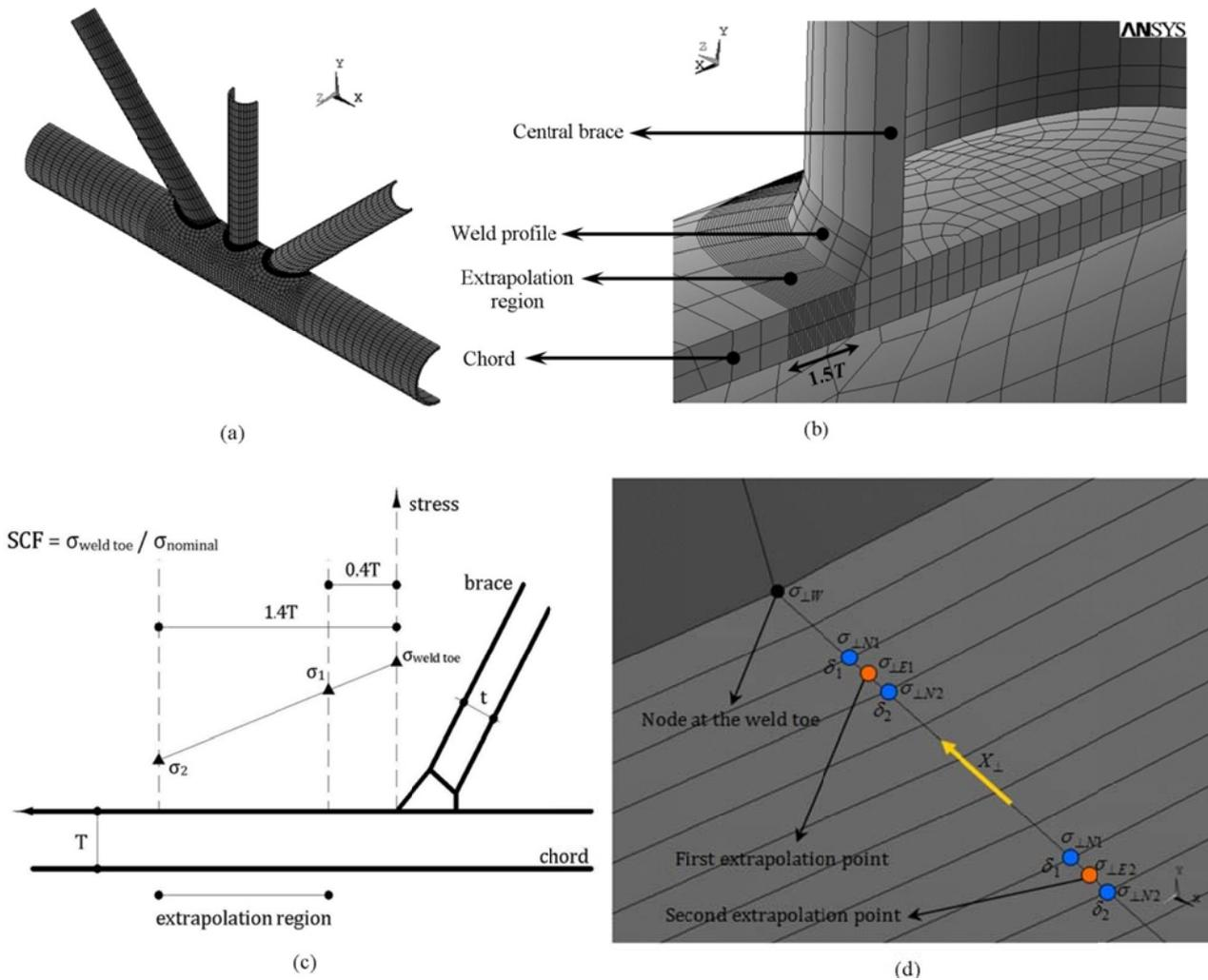
Fig. 2: (a) Global view of the generated mesh, (b) Mesh generated in the regions adjacent to the intersection, (c) Extrapolation method according to IIW-XV-E (1999), (d) Interpolations and extrapolations required to determine SCFs based on the stresses perpendicular to the weld toe
