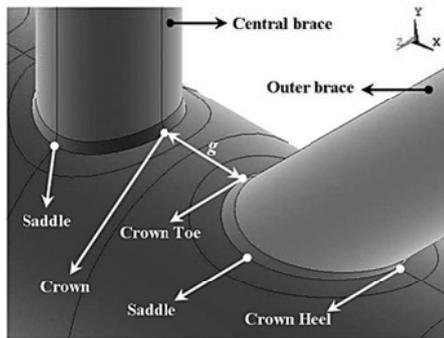
(c) Critical positions along the weld toe
