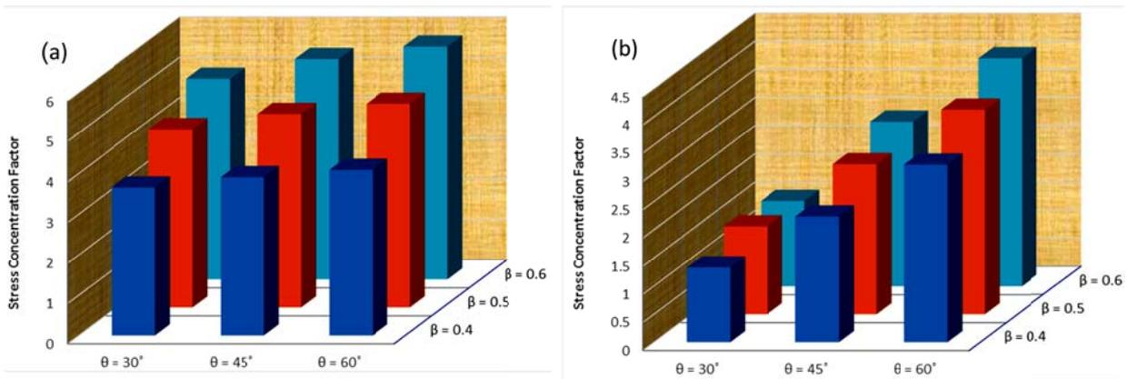
Fig. 7: Effect of the  $\theta$  on the SCF values at the saddle position under the 1st OPB loading condition ( $\tau = 0.4$ ,  $\gamma = 12$ ): (a) Central brace, (b) Outer brace
