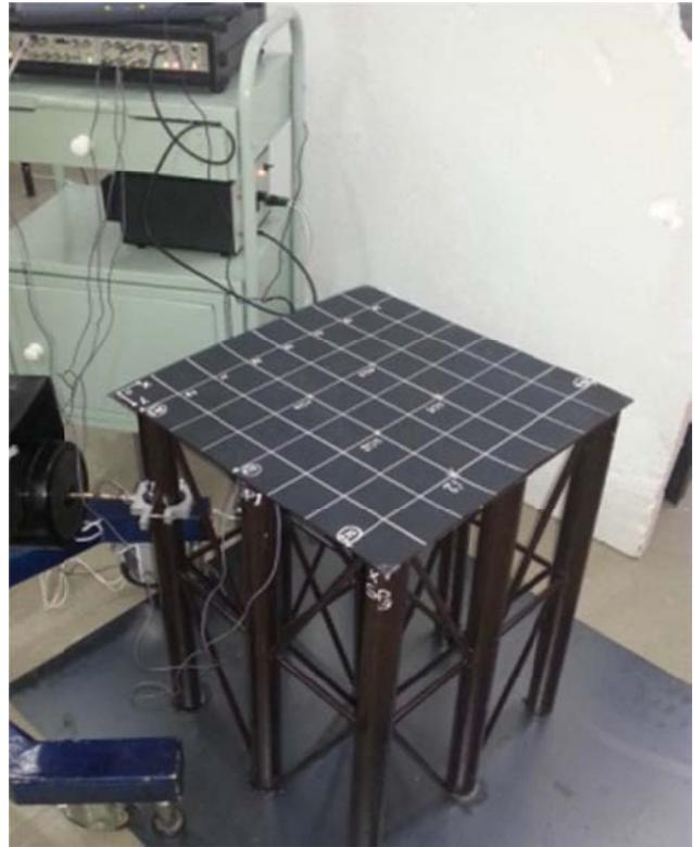
Fig. 1: Configuration of equipment used for experimental model analysis
