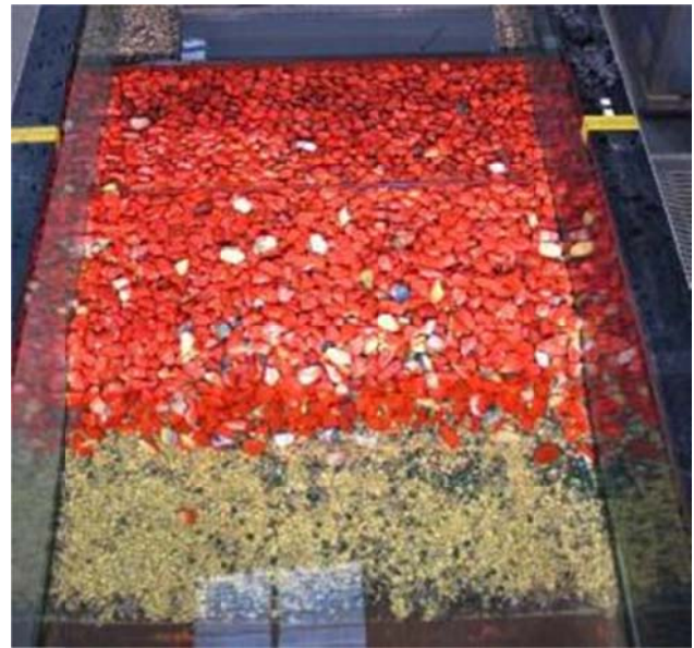
Fig. 16: Photo shows the third proposed section after the cyclone Gonu wave condition ( T_p=18.6s )
