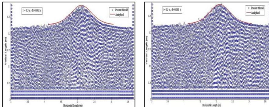
Fig. 1: Particle configurations and comparison of values computed by ISPH flow model and analytical surface profiles of solitary wave (horizontal and vertical scales units in meter)
