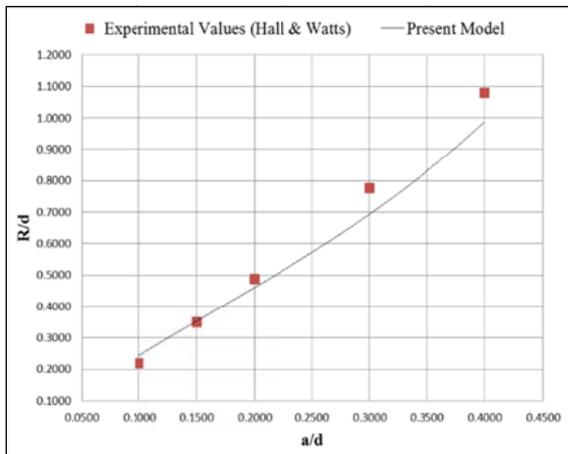
Fig. 4: Comparison between solitary wave run-ups on a slope with  $\alpha = 45^\circ$  computed by ISPH model and experimental based formula
