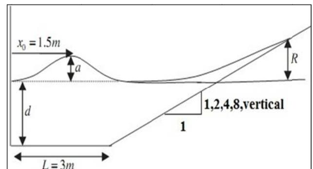
Fig 3: Geometry of Non-breaking solitary wave run-up
