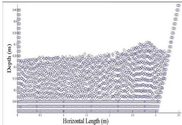
Fig. 5: Particle configurations at  $t = 0.8 \text{ s}$  for solitary wave run-up problem simulated by ISPH model
