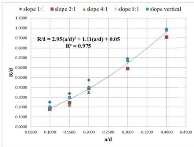
Fig. 6: Equation of solitary wave run-up rate by various amplitude against steep slopes
